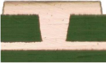
Just watch the results for good planarity. Sometimes the processing isn't nailed down and you can get either a indent or small bump over the filled via. The indent is probably most common when resin is used to fill the via. In either case, the bump or dip can lead to a less reliable assembly, especially with fine pitch BGAs and chip scale packages.
