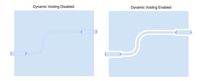
The clearance spacing between layout shapes and nets for various drawing layers is defined by constraint rules specified in the layout process file (LPF).
