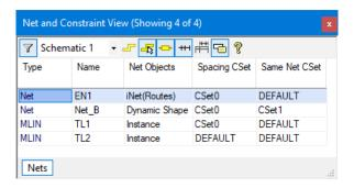
A new automatic net connectivity mode eliminates the need to manually select and associate shapes with nets. Shapes that overlay signal traces automatically inherit the net name of the signal trace.
