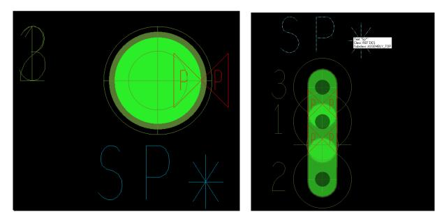
Open the board file and import the netlist from Capture. Place your components. You will notice in the next screenshot that the net short SP1 is placed and there are no DRC errors.
