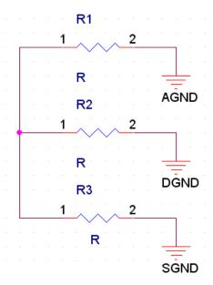
On each pin on the net short (SP1) you need to edit property and add the net names that you wish to short seperated by a colon. In this example the nets are DGND:AGND:SGND. You also need to ensure that you have a pcb footprint defined for this part.
