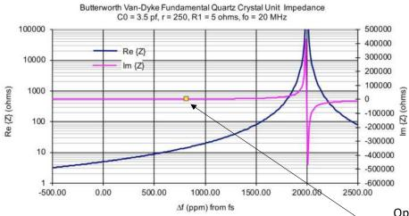
Operating frequency with input capacitance of 5 pf.
